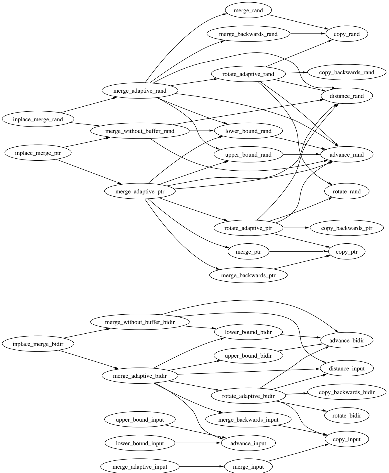
Figure 3: Call graph for inplace merge without overloading.
